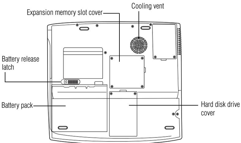
The **expansion memory slot cover** protects the slots where you insert additional memory. See “[Installing additional memory \(optional\)](#)” on page 57 for detailed information.
