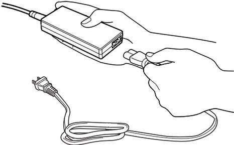
*Connecting the power cable to the AC adapter*
