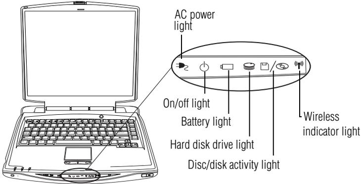
The system indicator lights are under a tinted panel and are visible only when the feature they represent is either on, or both on and active.
